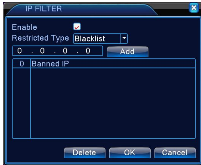
Pic 4.19 IP filter setup
