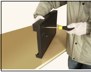
④fix the screw of hard disk
